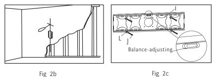
Using balance-adjusting system on the plate, make sure whether wall plate is installed balance. If not, then slide the wall plate let pointer level in the center position.
